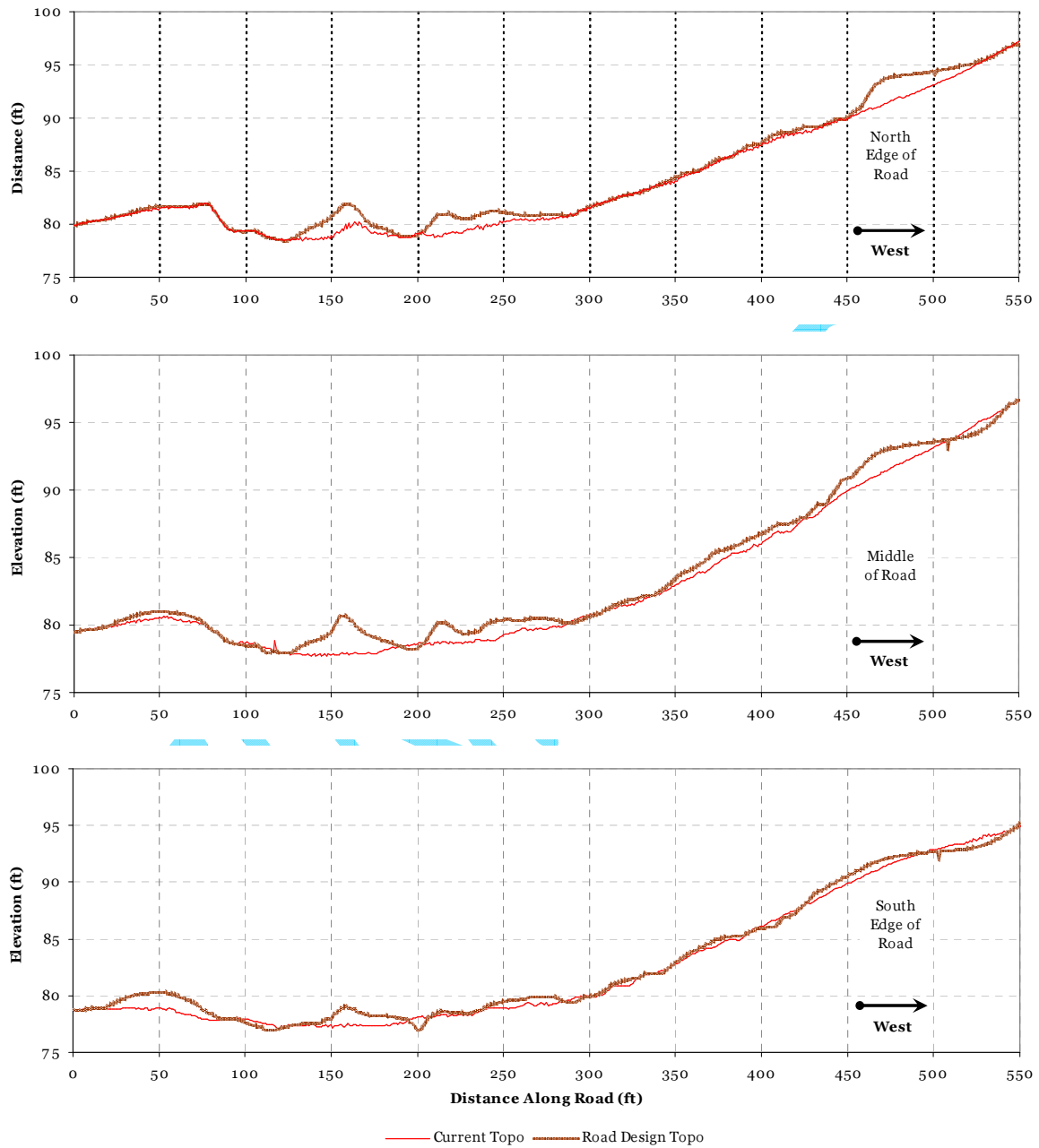
Figure D1. Longitudinal profile of road with before and after topography.
