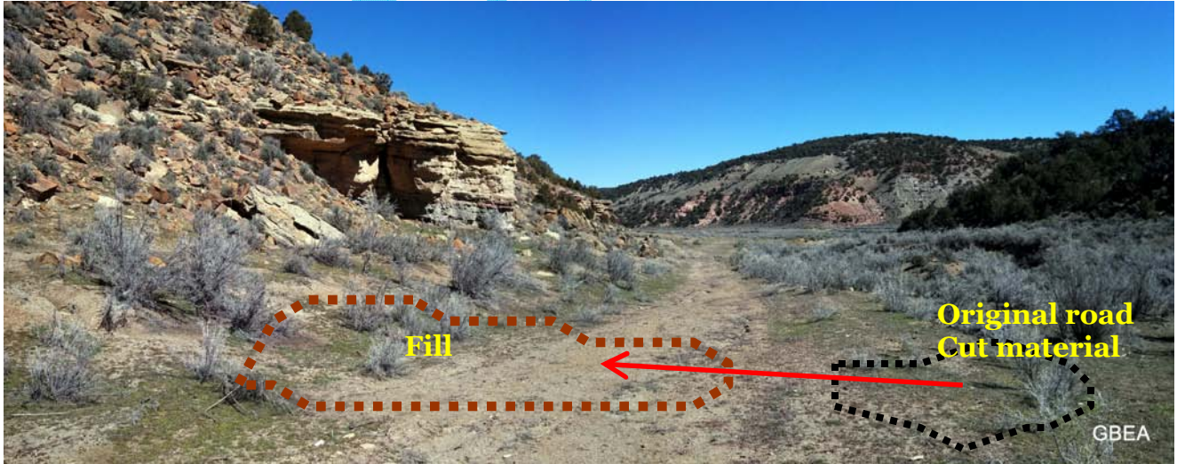
Photo 3. Original road cut material and fill diagram, superimposed upon access road section 4.
